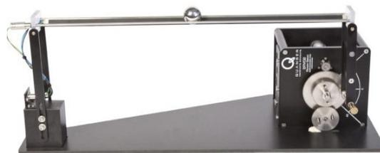
Figure 3.2: The ball-and-beam process used to evaluate the performance of the proposed control algorithms [8]
